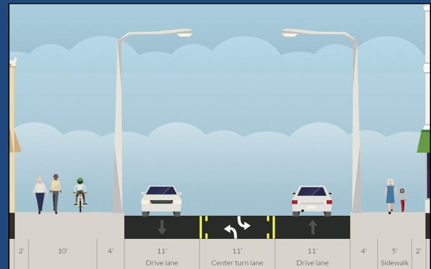
Two-11ft lanes and one 11ft continuous turn lane. A 10ft off-street shared use path on north side of street. One 5ft sidewalk on south side of street.
