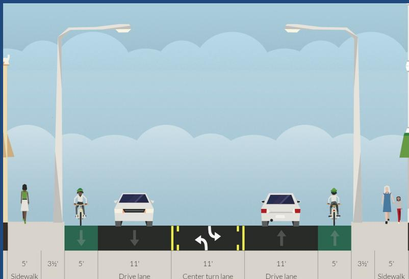
Two 11ft lanes and one 11ft continuous turn lane. The two 11ft travel lanes will include a striped 5ft bicycle lane on each side. Two 5ft sidewalks on both sides of street.
